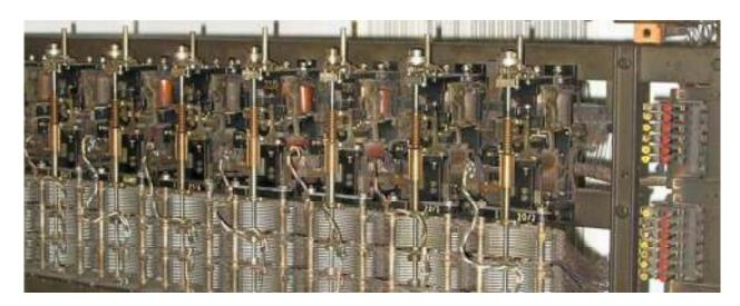
Voice call 1974. A rotary dial phone with battery in the central office on a mechanical switch would dial the 7 digit number of the person you want to call in the same area. The central office connects the lines
